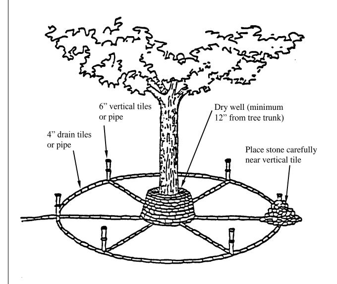
Figure AM-03-2 Typical Drainage Pipe Layout
