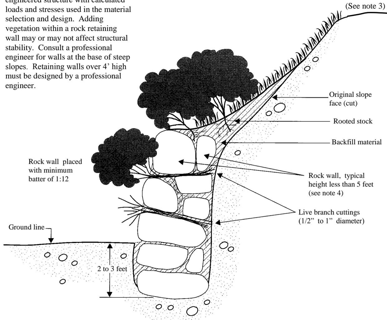
3. Limit height of slope and types of surcharged loads (such as buildings or traffic) above vegetated rock wall.
